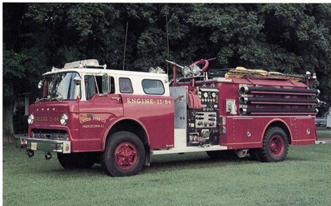
Unit 11-64 1978 Ford Ward LaFrance 1000 GPM Pumper
